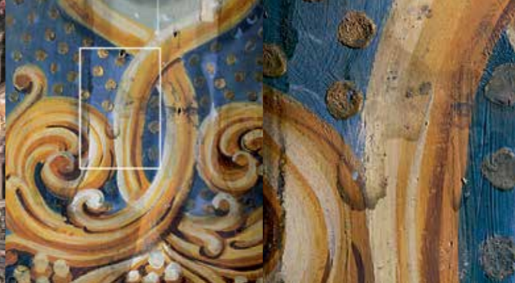
Findings showing the original colouring of the painting under the balcony of the northern trumpeters' loge
